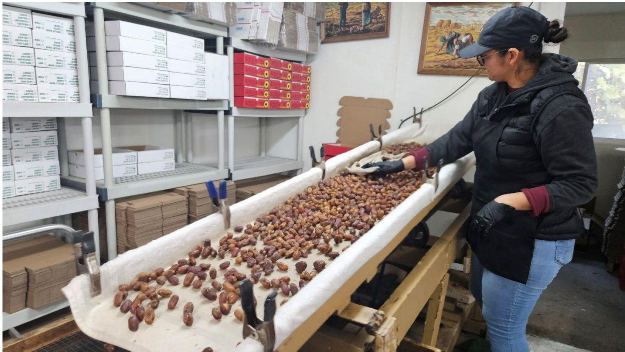
The date shaker removes excess debris from the dates prior to sorting and removing the pits.
